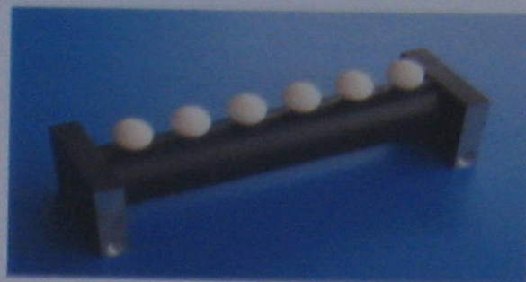
1) Ball bar (source: E. Trapet)
