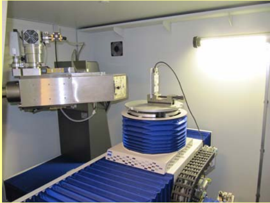
Figure 8: The CT-scanner at TI with the Yxl detector for measuring the stability of the beam
