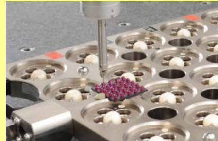
Figure 4: CT ball plate (left) and a setup for traceability transfer using a ball plate as part of the calibration procedure of the CT ball plate using CMM (right).
