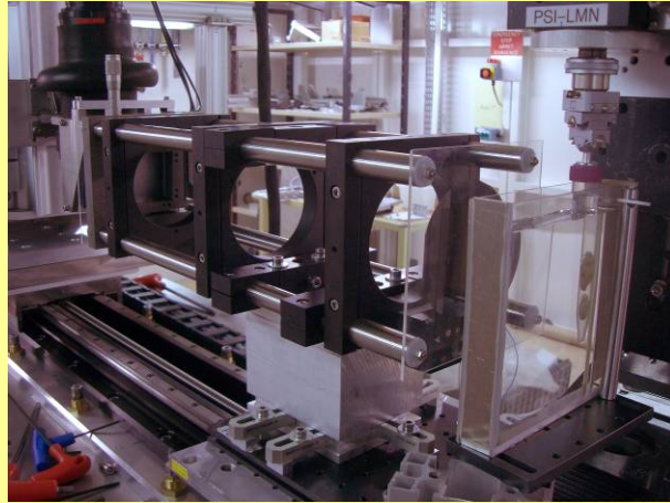
Figure 12: The grating interferometer used for phase-contrast tomography.
