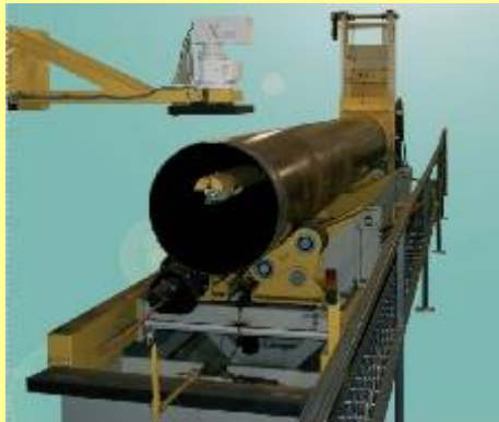
Figure 14: Pipe inspection machine, able to inspect steel pipes up to 25 m length (on the left); Crack in welding seen in steel pipe (on the right).
